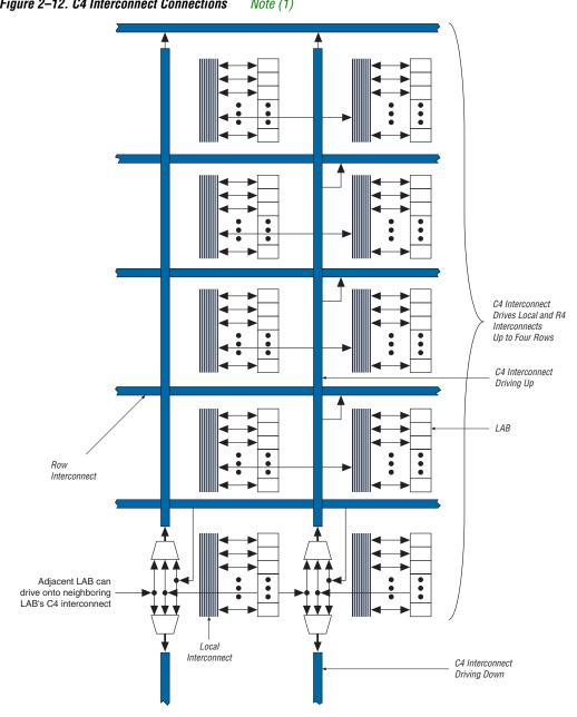
Figure 2–12. C4 Interconnect Connections Note (1)
