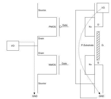
Figure 4–3. ESD Protection During Positive Voltage Zap
