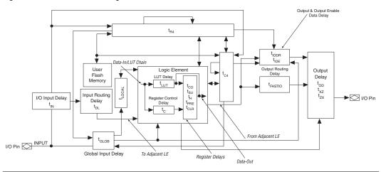
The timing characteristics of any signal path can be derived from the timing model and parameters of a particular device. External timing parameters, which represent pin-to-pin timing delays, can be calculated as the sum of internal parameters. Refer to the chapter on *Understanding Timing in MAX II Devices* for more information.
