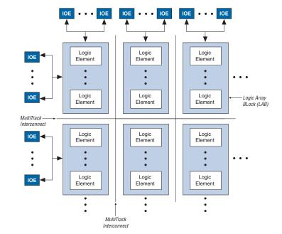
Figure 2–1. MAX II Device Block Diagram
