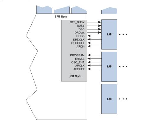
Figure 2–17. EPM570, EPM1270 & EPM2210 UFM Block LAB Row Interface
