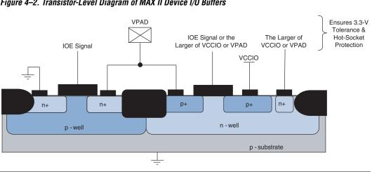
The CMOS output drivers in the I/O pins intrinsically provide electrostatic discharge (ESD) protection. There are two cases to consider for ESD voltage strikes: positive voltage zap and negative voltage zap.
